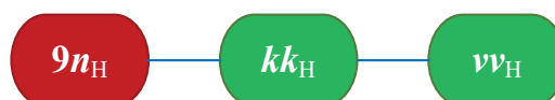
Fig. 2. Structure of Note-On MIDI message (where: n – number of MIDI channel, kk – number of MIDI note, vv – velocity value)
