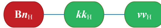
Fig. 3. Structure of Control Change MIDI message (where: n – number of MIDI channel, kk – controller number, vv – value)
