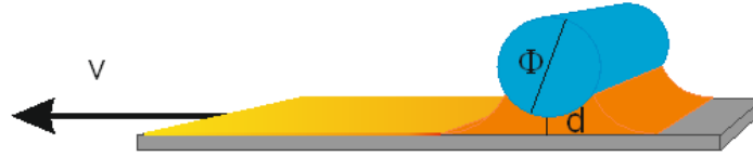
Figure 22. Schematic presentation of the coating process, the wet film thickness depends on the coating bar diameter \Phi , the distance between the bar and the substrate d , and the velocity v [176].
