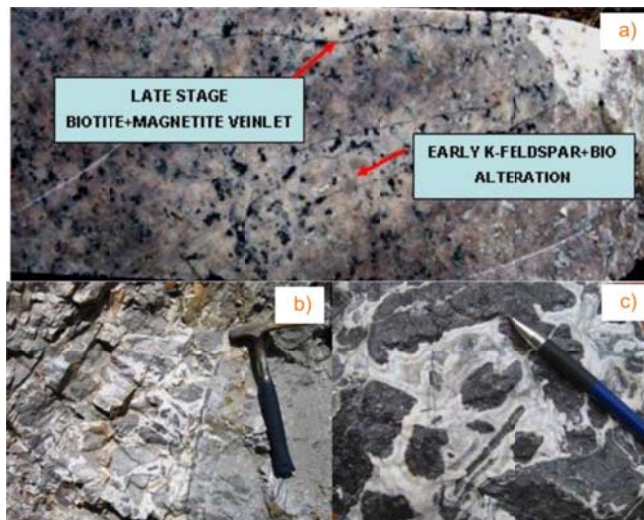
Fig. 7.11. a) Upper Nam Dich drill core, alteration and mineralization in syenite; b, c) Mineralized breccia, Can Ho mine (Photographs from Howell et al. , 2007)
